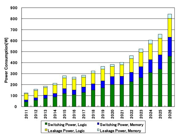
Figure SYSD11 SOC Consumer Stationary Power Consumption Trends
