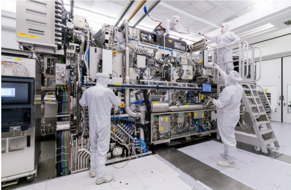
Figure 10-1 ASML Latest Extreme Ultraviolet Photolithography Exposure Tool. 79
